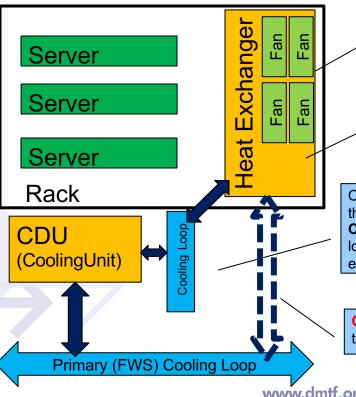
The heat exchanger model includes a Chassis with a ThermalSubsystem that describes the Fans
